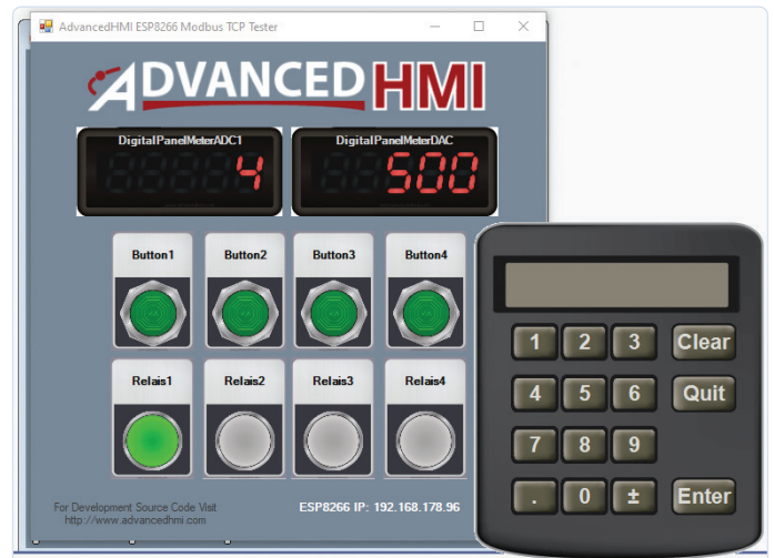
Figuur 2. De AdvancedHMI-software genereert HMI's.
