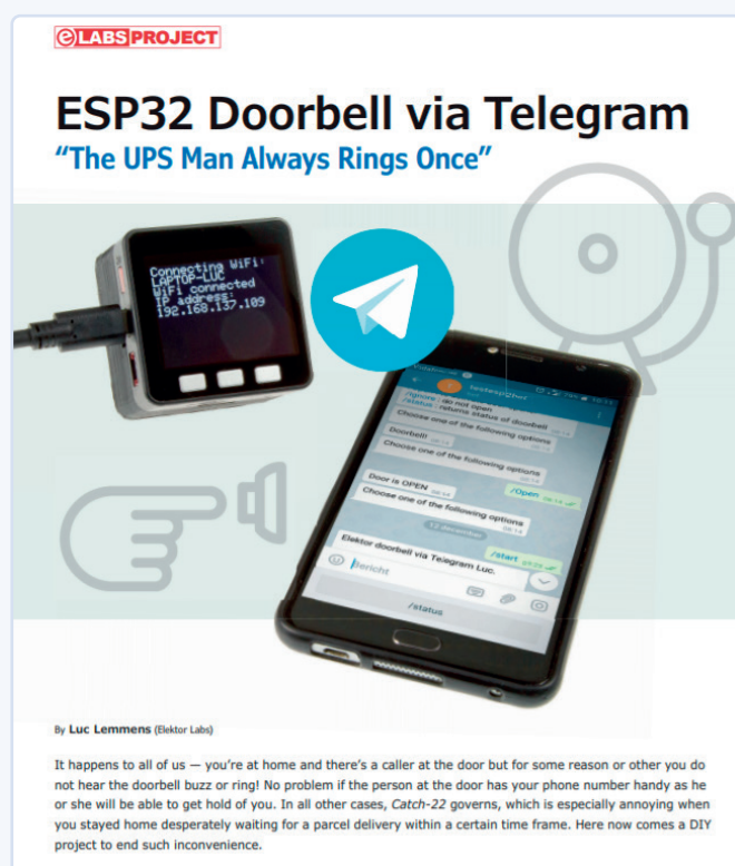
Figure 1: In early 2020, Elektor engineer Luc Lemmens presented a ESP32 doorbell project that many will find useful. When the doorbell rings, the circuit can send a message to your smartphone or computer. (Elektor March & April 2020)
