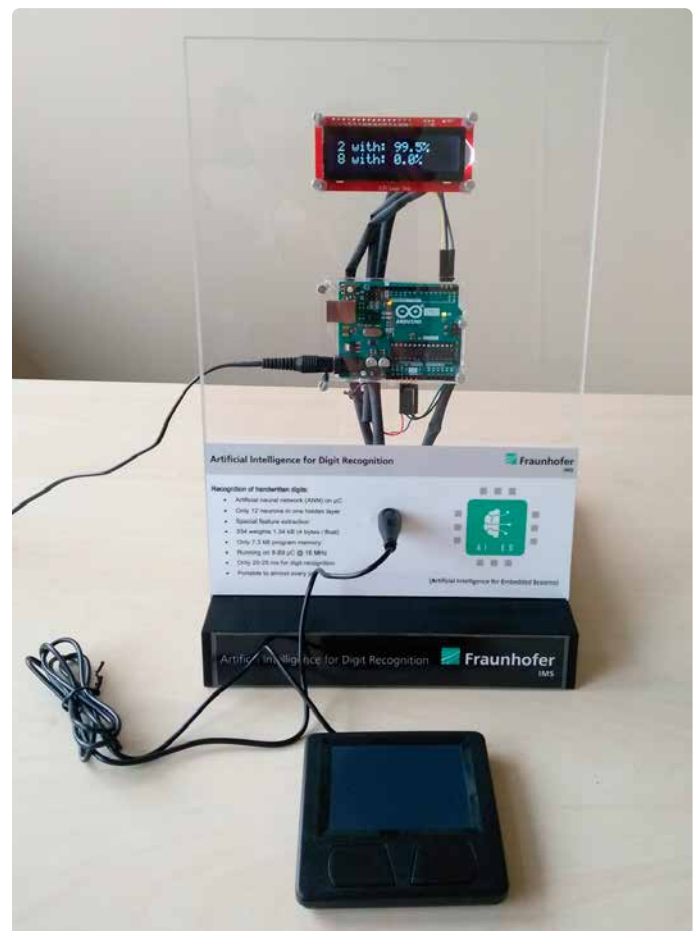
Figure 5: The AIFES from Fraunhofer Institute for Microelectronic Circuits and Systems runs handwriting recognition on an Arduino UNO. (Copyright: Fraunhofer IMS)
