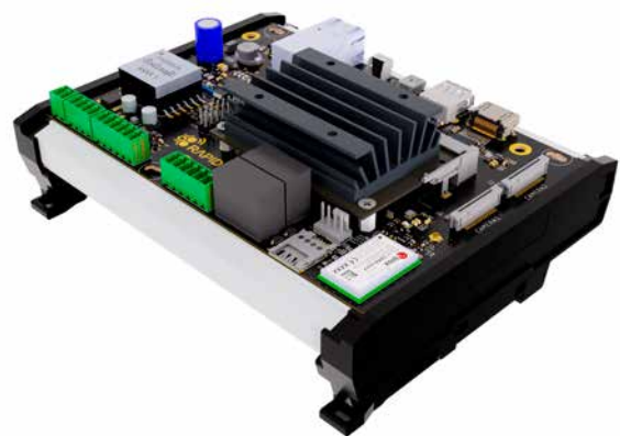
Figure 4: Low-latency ML is enabled by solutions such as RapidLab's Edge AI Gateway featuring NVIDIA's Jetson Nano. (Source: rapidLAB.io)
