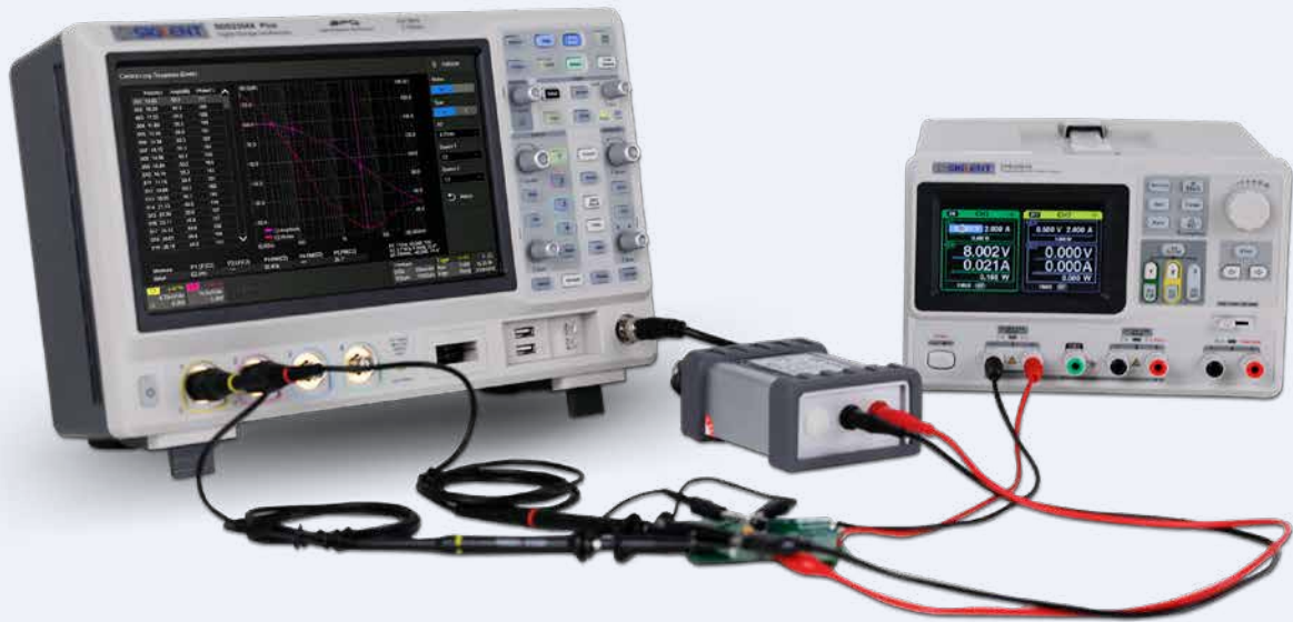
Figure 1: Bode diagrams are typically used to measure the phase and gain margin of feedback systems.
