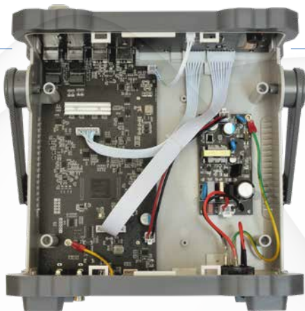
Figure 4: The inside of the PSG9080. At the heart is an Xilinx Spartan-6, in the middle on the large circuit board. The power supply is on the right.
