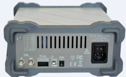
Figure 2: The back of the generator, with a "real" mains switch and a USB connection, among others.
