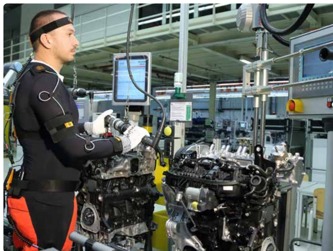
Figure 1: Motion digitizer unit collecting data.
