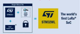
The STMicroelectronics STM32WL range of MCUs is integrating LoRa, SigFox and legacy sub 1-GHz with a single or two core Cortex-M solution into a single die for lowest power consumption.
