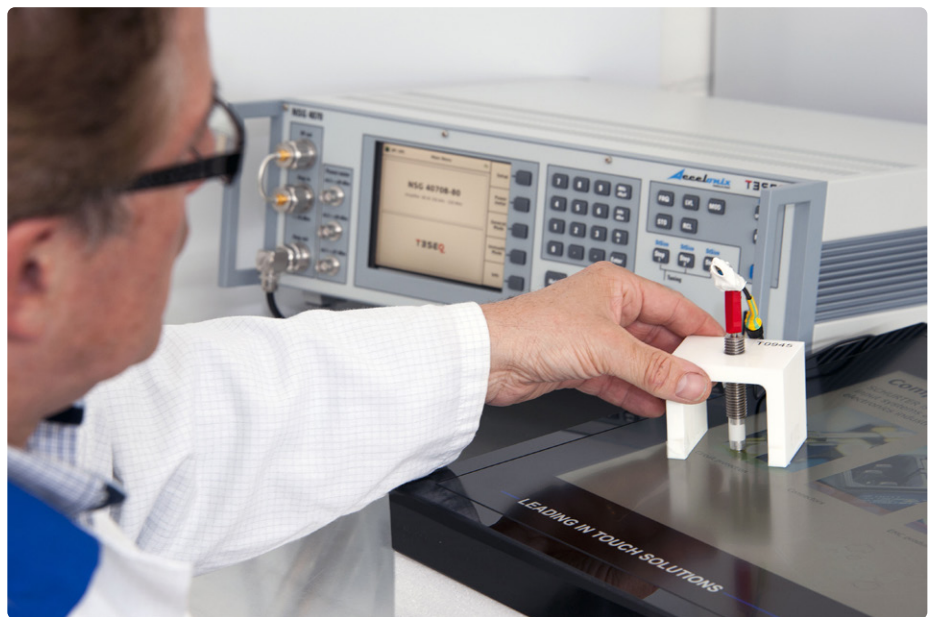
Figure 2: Performing a conducted immunity EMC test.
