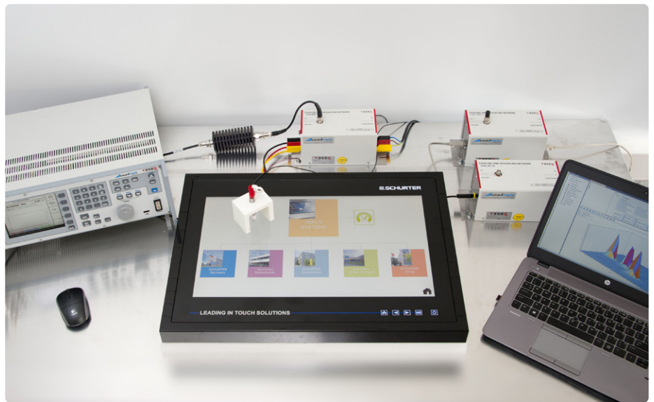
Figure 1: Conducted immunity EMC test setup for touchscreens.
