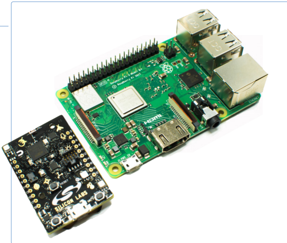
Figure 1: UrsaLeo IoT hardware — comprising a Thunderboard 2 module and a Raspberry Pi 3B+.
