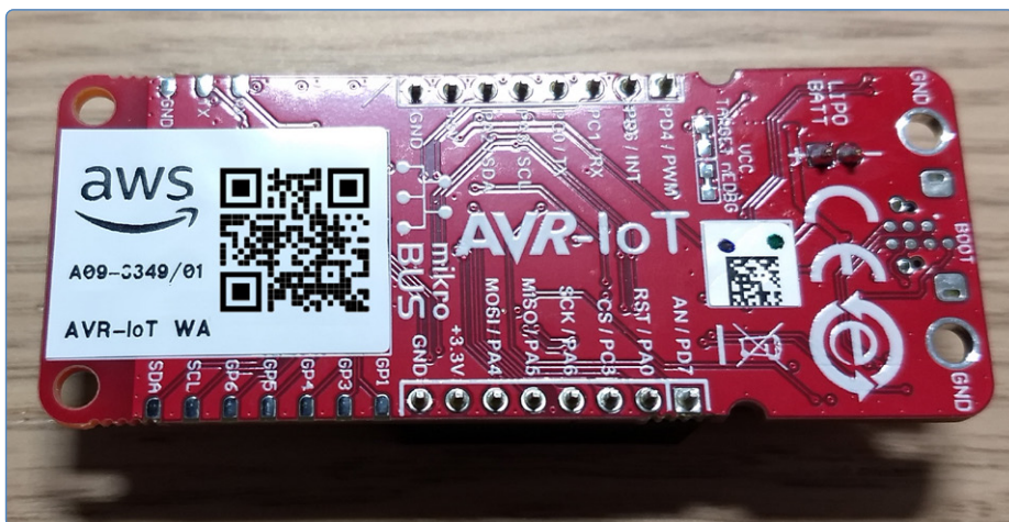
Figure 6: The backside of the IoT WA Development Board showing pin labels.
