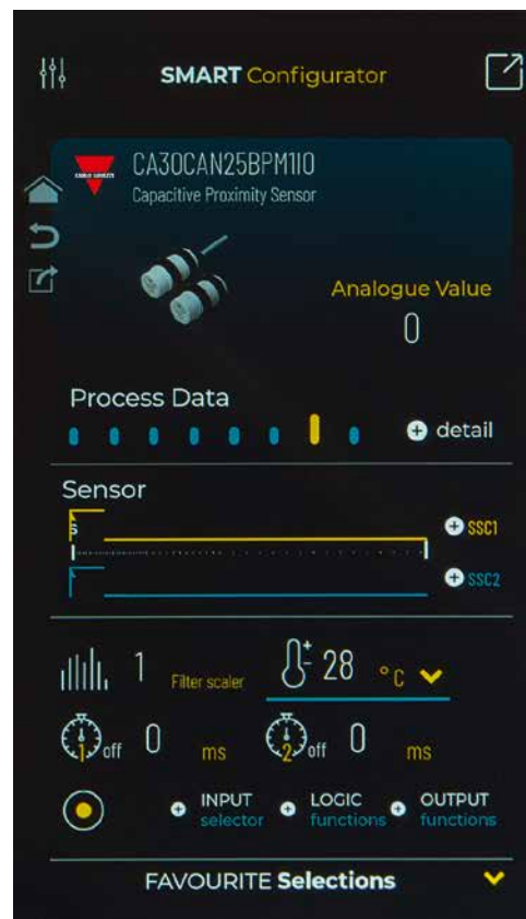
Figure 2: Carlo Gavazzi's Smart Configurator gives service technicians access to parameters, process data and diagnostic information from sensors and enables on-site adjustments.
