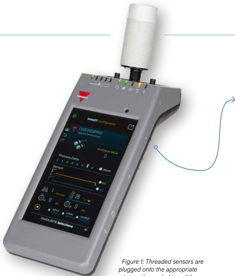
Figure 2: Carlo Gavazzi's Smart Configurator gives service technicians access to parameters, process data and diagnostic information from sensors and enables on-site adjustments.
